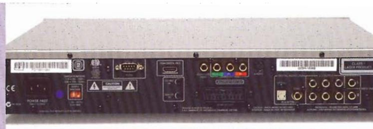
Back-panel connections include an RS232 port for system integration plus 5.1 phonos for multichannel audio support
